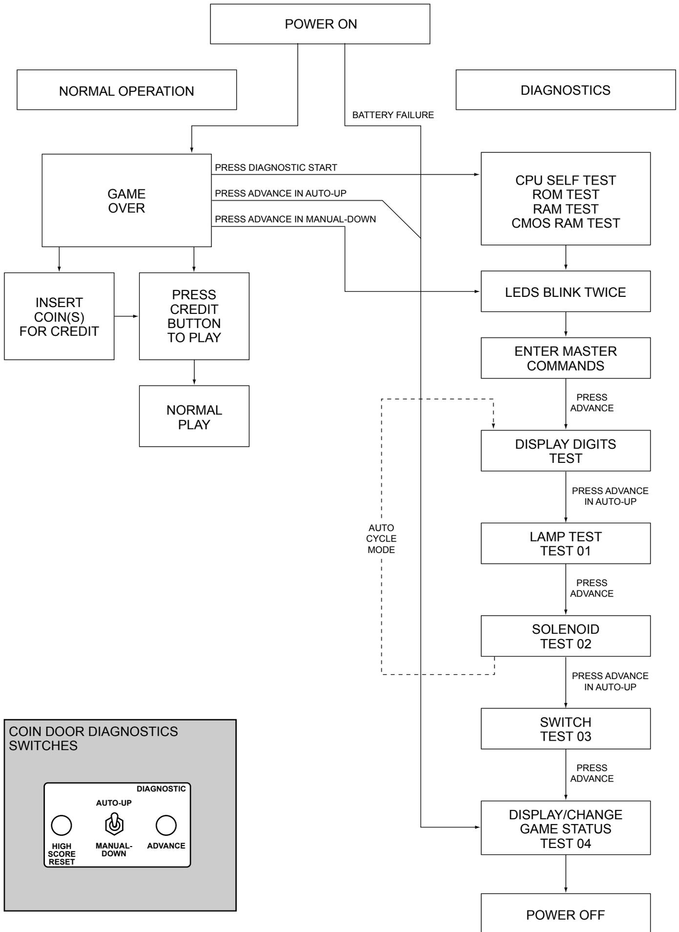
Figure 3. Normal Operation and Diagnostic Flow Chart
