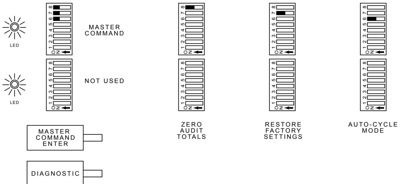
3. Momentarily depress the ADVANCE pushbutton. Function 01 is indicated on the number of credits display and the number of coins through the left chute (closest to coin door hinge) is indicated on the Player 1 display.
